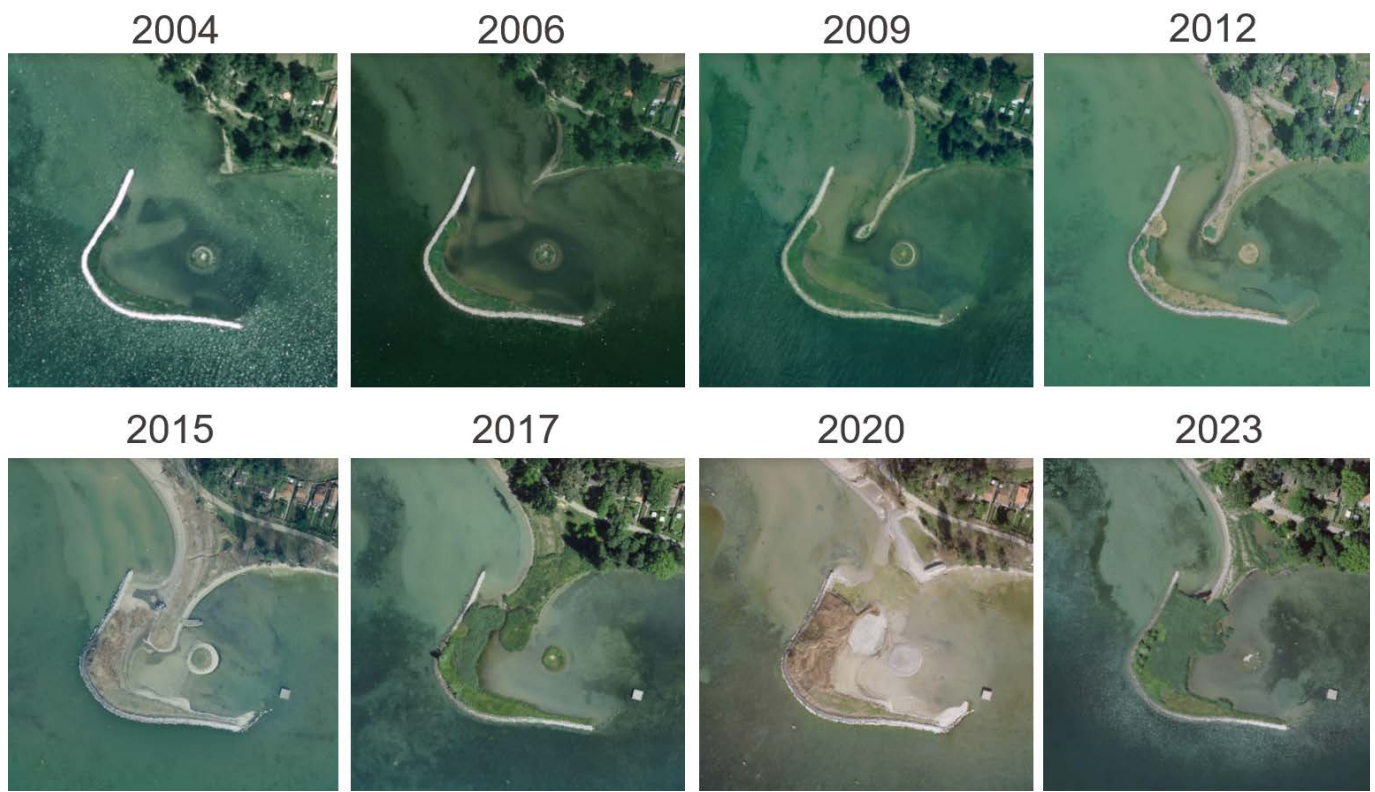
Figure 6: The evolution of the Préverenges Bird Island since its formation in 2002. The formation of a spit that developed into a tombolo. Despite the dredging that was clearly visible in 2020, the tombolo quickly reformed, although somewhat narrower.
